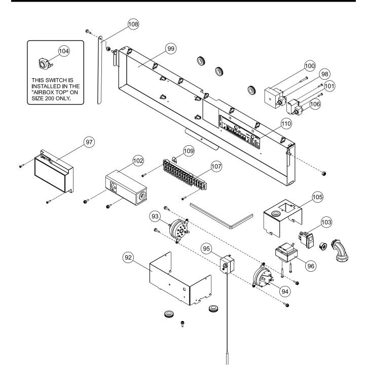
Figure 24. Control Panel Components.
